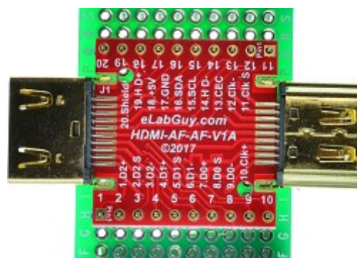
Figure 2: Example of connecting the HDMI-AF-AF-V1A on a proto PCB (Note: This picture only shows the pins spacing, actual use may not be used on a breadboard)
